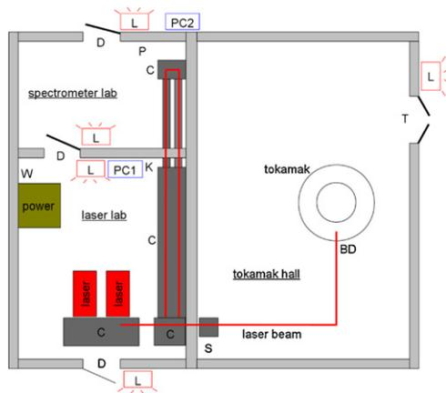
Fig. 2. Layout of key elements of the TSP system: C—box covers, D—door contacts, L—warning lights, PC1, 2—control PC, P—push button to confirm spectrometer laboratory check, W—cooling water flow, K—operators keys, S—beam shutter, BD—beam dump, T—tokamak hall door.
